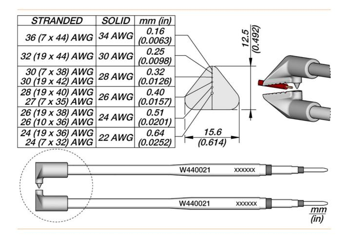
• especially for the stripping of high temperature wire insulation made of thermostable materials like Teflon, Kapton, silicone rubber etc.
