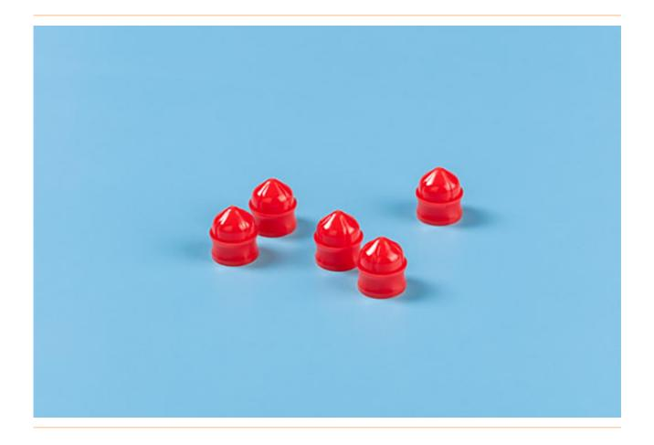
A piston is inserted into the syringe barrel after it has been loaded with fluid to ensure uniform dispensing, prevent dripping, and eliminate waste by wiping barrel walls clean as fluid is dispensed. Optimum pistons are molded from high-density polyethylene. For use with mechanical dispensing equipment.
