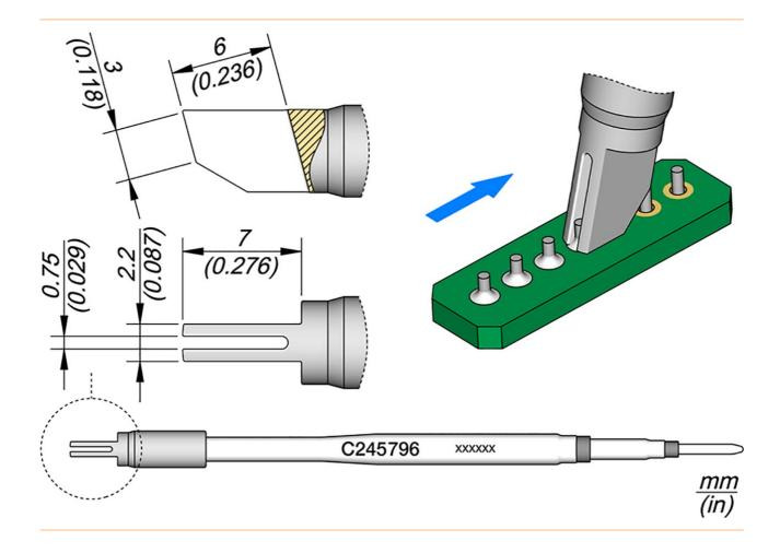
Soldering tips series C245 for soldering iron T245 (formerly AD-2245). They are suitable for general soldering purposes. Sleep and sleep mode in the clipboard.
