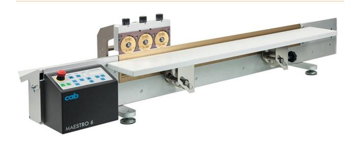
Separation of pre-scored PCBs up to 1,500 mm length with minimum stress on the components
