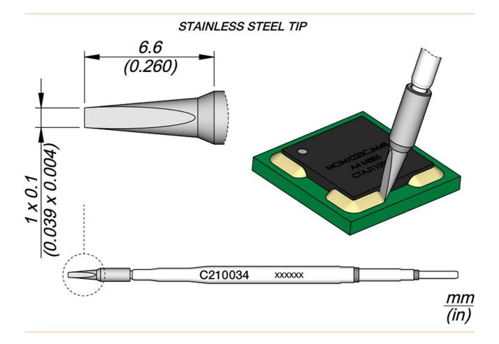
This cartridge with a stainless steel tip is perfect to remove reworkable underfill encapsulants.
