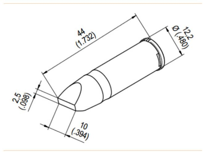
• Suitable for soldering iron HighPower-Tool (0240CDJ) of soldering station i-CON Vario HP in version 0ICV2000HP
