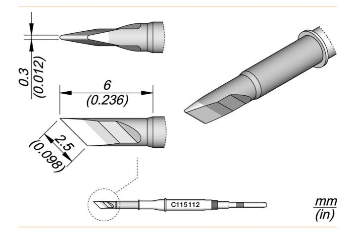
The C115 series soldering tips are suitable for soldering and repairing very small components. These are compatible with NT115-A, NP115-A and AN115-A Nano soldering handpieces.
