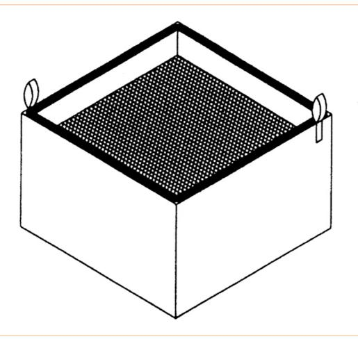
• Particle filter H13 and broadband gas filter (50 % activated carbon / 50 % chemisorb)
