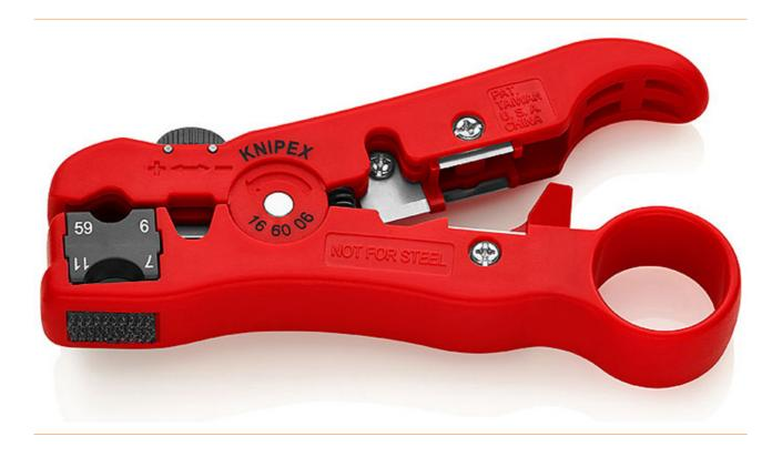
Stripping tool for coaxial and data cables Universal stripping tool for coaxial cables RG 59, RG 6, RG 7, RG 11. For stripping outer sheath, shield and insulation in one operation. Adjustable stripping blade for data cables. Two stripping blades for cutting and stripping telephone ribbon cables (4P/6P/8P) in one operation. Integrated blade for cutting data cables. - Cable type: RG 59, RG 6, RG 7, RG 11
