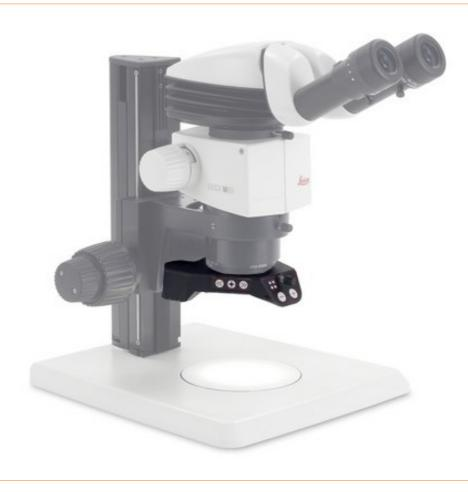
• produces a bright and uniform illumination of the sample with constant colour temperature and a large field of view
