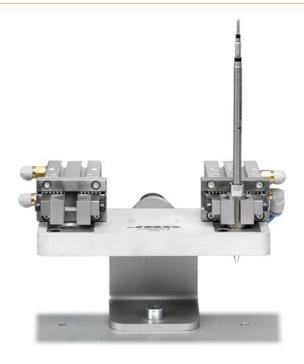
This Cartridge Stand is designed to be used in combination with the new Cartridges R245. The Cartridges Stand mechanism works with compressed air to fix and release the cartridges automatically. In order to facilitate the automatic cartridges fixation and release, the position of the Stand can be adjusted by pivoting up to 35° in both directions and can therefore be optimally adapted to the working position. It can be combined with the Automatic Soldering Iron TRA245 and the Control Box UCR245.
