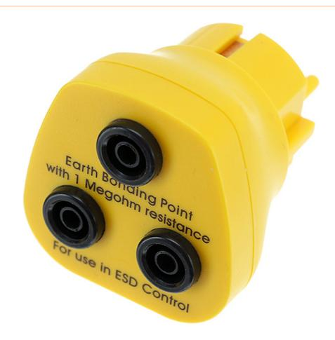
The Safeguard ESD grounding plug is designed to protect electronic equipment and components from damage caused by electrostatic discharge. The plug has 3 x 4mm banana jacks and offers a 1 megohm safety resistor per connection. With the help of the plug sockets you can work ESD-safe and avoid damage to sensitive components. The 1 megohm safety resistor ensures that static electricity is dissipated effectively and safely. The yellow design of the connector helps to quickly identify and access it.
