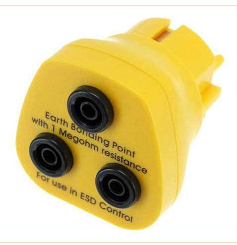
The Safeguard ESD grounding plug is designed to protect electronic equipment and components from damage caused by electrostatic discharge. The plug has 3 x 4mm banana jacks and offers a 1 megohm safety resistor per connection. With the help of the plug sockets you can work ESD-safe and avoid damage to sensitive components. The 1 megohm safety resistor ensures that static electricity is dissipated effectively and safely. The yellow design of the connector helps to quickly identify and access it.
