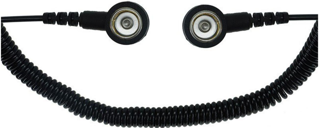
The ESD spiral cable from Safeguard is an important component for earthing people in the ESD zone (EPA) to protect electronic devices and components from electrostatic discharge. The leakage resistance is 2 Mohm. The length of the cable of 3.6 meters allows flexible working without restricting freedom of movement. The ESD spiral cable in black has 2x 10 mm press studs. The colouring makes it easy to see the cable at all times and in different lighting conditions.
