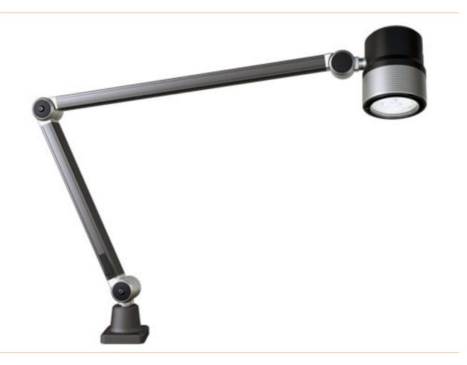
Maintenance-free LED technology. Powerful high power LEDs for maximum light. With wide beam light characteristic. Continuous and flicker-free dimming (switchable). Robust aluminium housing with solid safety glass cover. Viton seal for a high degree of protection. Chemically resistant to many media such as oils or cooling lubricants. Precisely adjustable boom. Connection to machine voltage.
