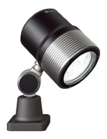
Maintenance-free LED technology. Powerful high power LEDs for maximum light. With wide beam light characteristic. Robust aluminium housing with solid safety glass cover. Viton seal for a high degree of protection. Chemically resistant to many media such as oils or cooling lubricants. Precisely adjustable rod end. Direct connection to machine voltage.
