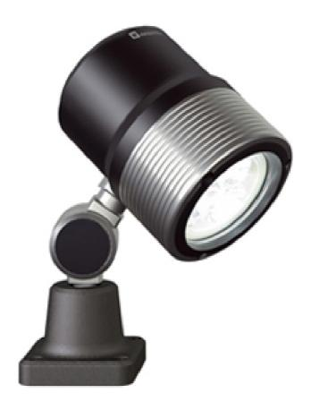
Maintenance-free LED technology. Powerful high power LEDs for maximum light. With narrow beam light characteristic. Robust aluminium housing with solid safety glass cover. Viton seal for a high degree of protection. Chemically resistant to many media such as oils or cooling lubricants. Precisely adjustable rod end. Direct connection to machine voltage.
