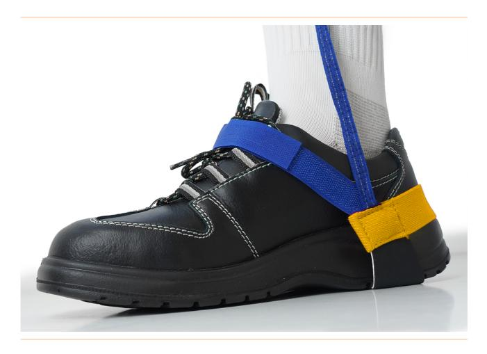
The ESD heel strap from Safeguard is an important accessory for correct personal grounding. It has a leakage resistance of 1 MOhm and a Velcro closure. The heel strap is designed to dissipate static electricity from the feet, preventing damage to electronic equipment and components. The 1 MOhm leakage resistance ensures that static electricity is dissipated effectively and safely. The tape is blue/yellow and suitable for street shoes with flat heels.
