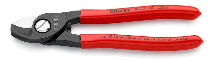
For cutting copper and aluminium cables, solid and stranded. Cuts smoothly and cleanly without crushing. Not suitable for steel wire and hard-drawn copper conductors. Hardened cutting edges with precision grinding. Easy cutting with one-hand operation. With clamping protection. Adjustable screw joint, self-locking. - Shape: 1 - Cutting value Cu-cable, stranded: 50mm² - Cutting value Cu-cable, stranded: Ø 15mm - AWG: 1 / 0
