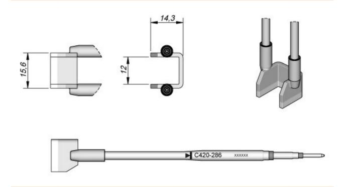
The C420 tip series are suitable for soldering and desoldering SMD components. The soldering tips are compatible with the thermo tweezers HT420 and are sold separately.
