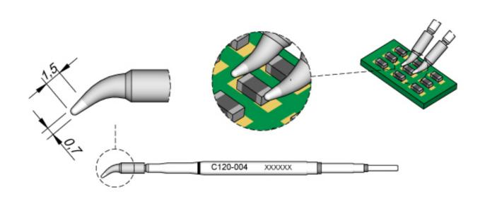
The C120 series soldering tips are suitable for PA120 micro tweezers. These can be used for soldering and desoldering chip components or dual-in-line. The tips are sold separately.
