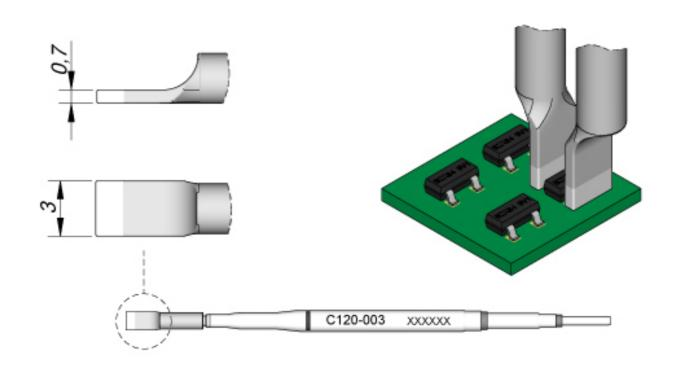
The C120 series soldering tips are suitable for PA120 micro tweezers. These can be used for soldering and desoldering chip components or dual-in-line. The tips are sold separately.
