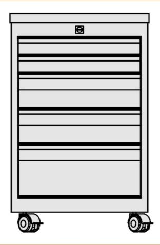
The mobile drawer unit F0 is characterized by its 4 conductive castors with a diameter of 52 mm, 2 of which are lockable. With a height of 670 mm and a depth of 540 mm, it offers versatile storage space. The lid is directly coated with ESD (electrostatically dissipative) to protect sensitive electronic components. A practical and mobile storage element for a wide range of applications.
