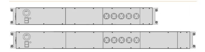
Electrical connection strips are space-saving solutions for office environments. With a sturdy sheet metal housing and height-adjustable mounting, they offer flexibility. Modules can be easily replaced and extended. The WINSTA plug-in connector system simplifies mains connection and wiring. With emergency stop, circuit breaker and five Schuko sockets (D), they are ideal for desk widths of 1230 mm.
