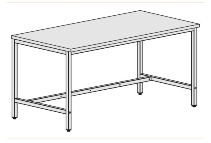
The reinforced design of the ESD work table Basic by Karl fulfils all standards which are prescribed for an ESD-compliant workplace in an EPA in order to ensure safe working with sensitive electronic components. Thanks to the reinforcing struts on the table frame, the table top can be loaded with up to 200 kg of uniform surface load.
