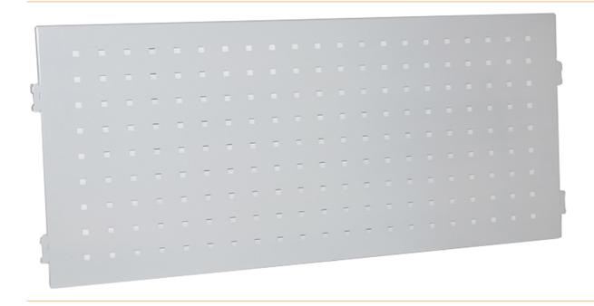
The hole size is  $9 \times 9$  mm, distance from hole centre to hole centre 38 mm. Fastening to the upright grid tube profiles.
