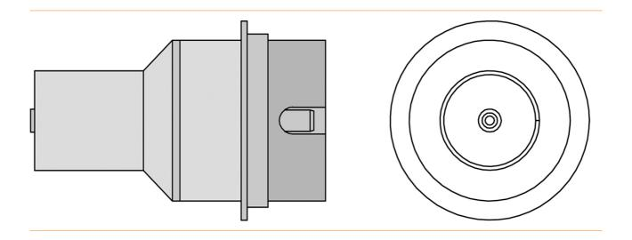
has an integrated preheating plate for preheating the components by means of contact heat. Around the plate there are air outlet slots for the hot air of approx. 1 mm width.
