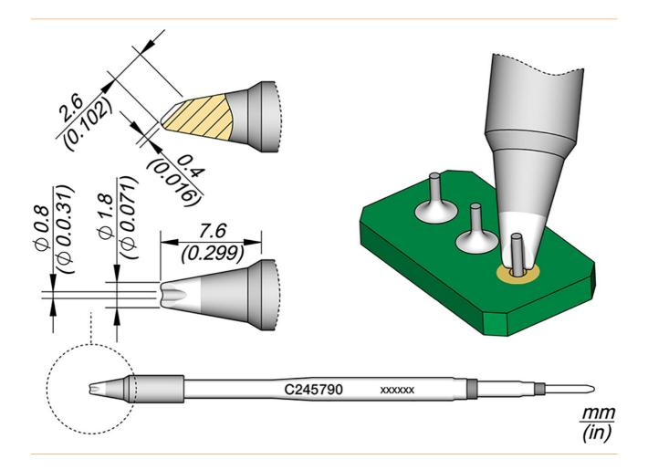
Soldering tips series C245 for soldering iron T245 (formerly AD-2245). They are suitable for general soldering purposes. Sleep and sleep mode in the clipboard.
