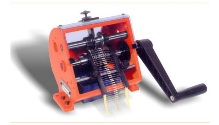
Cutting and bending machine for belted, axial components for push-in assembly
