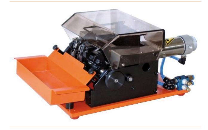
Cutting, stamping and bending device for axial components manual operation
