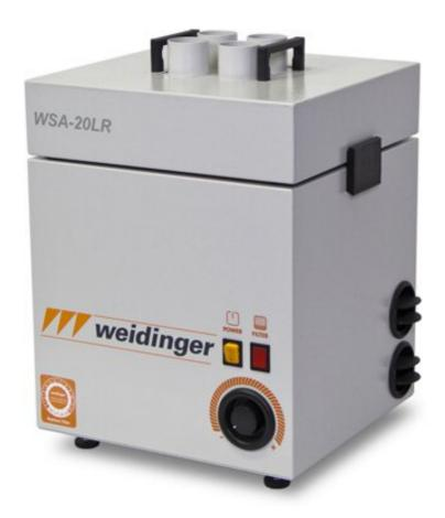
The WSA-20LR extraction unit for solder fumes has 4 extraction ports with an outer diameter of 50 mm (top), 4 adjustable blow-out gills (both sides, bottom), an optical filter indicator and a volume flow controller including a constant negative pressure control.
