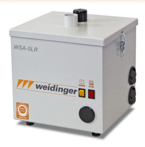
The WSA-5LR extraction unit for solder fumes has 2 extraction ports with an outer diameter of 50 mm (top), 4 adjustable blow-out gills (both sides, bottom) and an optical filter indicator.
