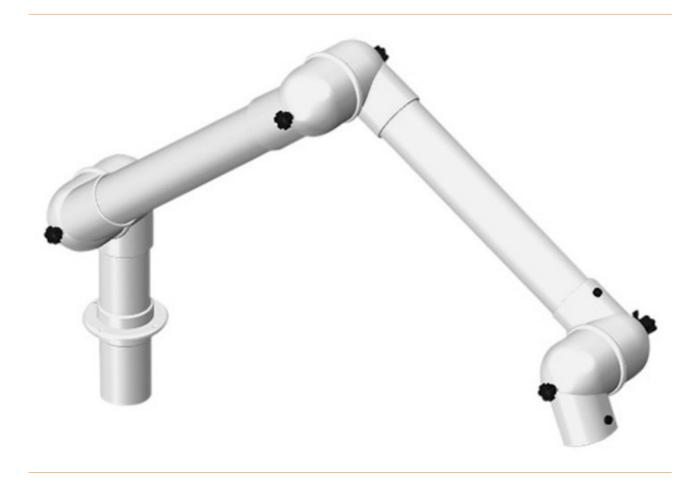
The Alsident System 63 is chemically resistant and therefore particularly suitable for use in aggressive environments such as laboratories in the chemical, pharmaceutical and food industries. The recommended air volume is  $60 - 120 \, \text{m}^3/\text{h}$  and the pipes have a diameter of  $63 \, \text{mm}$ .
