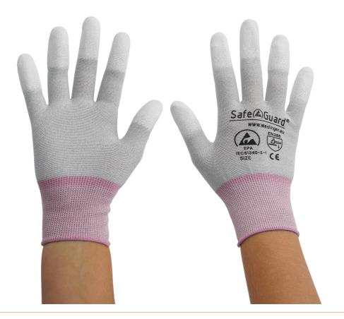
The ESD glove with coated fingertips is made from 80% nylon and 20% carbon. It is also seamless and particularly comfortable to wear. The antistatic glove can be washed and has a leakage resistance of  $10^{7}$ - $10^{8}$  Ohm.
