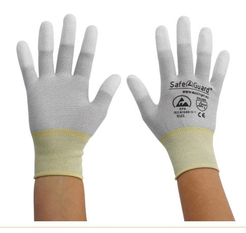
The ESD glove with coated fingertips is made from 80% nylon and 20% carbon. It is also seamless and particularly comfortable to wear. The antistatic glove can be washed and has a leakage resistance of 10<sup>7</sup>-10<sup>8</sup> Ohm.
