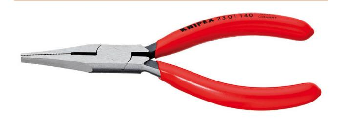
Flat nose pliers with cutting edge Suitable for finer gripping and cutting work. Flat, long jaws, thin tapered. Cutting edges additionally induction hardened, cutting edge hardness approx. 60 HRC. - Cutting value medium hard wire (diameter): Ø 1,6mm - Cutting value soft wire (diameter): Ø 2,5mm - Jaw thickness (T1): 7,0mm - Tip width (E): 3,0mm - Tip thickness (D1): 4,5mm - Jaw length (L3): 35,0mm - Head width (W3): 12,5mm
