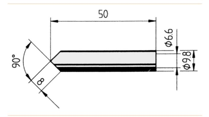
• Continuous soldering tip, straight, bevelled on both sides, 8.0 mm wide, with ERSADUR-LF coating (lead-free soldering) for increased service life.
