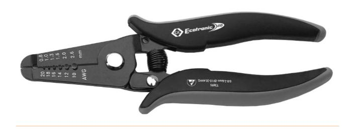
• For safe and gentle stripping of fine, insulated cables with a solid core in applications where damage caused by electrostatic charge must be avoided at all costs Six pre-set pairs of cutting edges for stripping fine, insulated cables with solid core, 0.8, 1.0, 1.3, 1.6, 2.0 and 2.6mm (10
