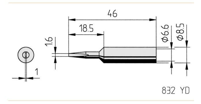
• Continuous soldering tip, straight, chisel-shaped, 1.6 mm wide, with ERSADUR-LF coating (lead-free soldering) for increased service life.
