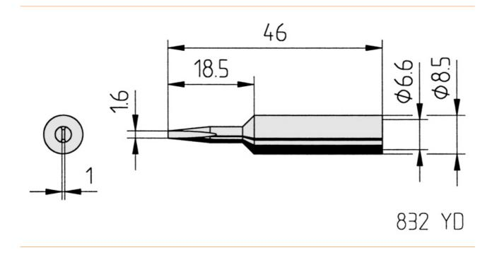
Continuous soldering tip, straight, chisel-shaped, 1.6 mm wide, with ERSADUR coating.
