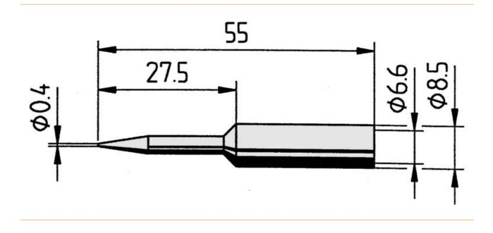
• Continuous soldering tip, straight, extended, pencil tip, 0.4 mm diameter with ERSADUR-LF coating (lead-free soldering) for increased tool life.
