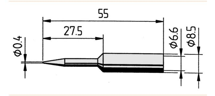
Continuous soldering tip, straight, pencil tip, 0.4 mm diameter, with ERSADUR coating.
