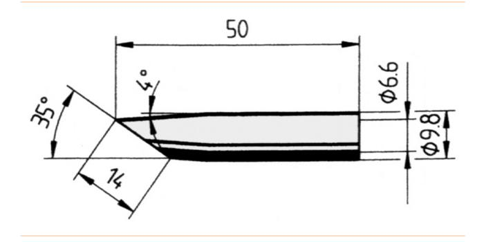
• Continuous soldering tip, straight, bevelled 35° angle, 14.0 mm wide, with ERSADUR-LF coating (lead-free soldering) for increased service life.
