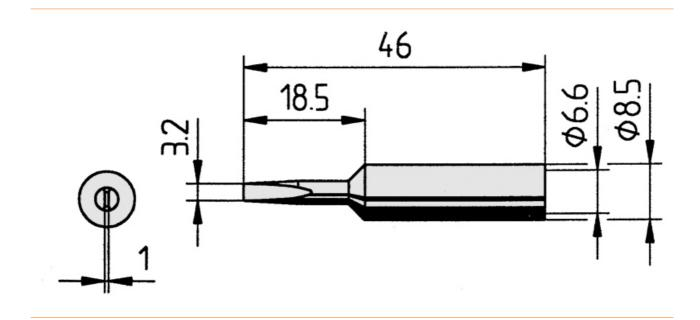
Continuous soldering tip, straight, chisel-shaped, 3.2 mm wide, with ERSADUR coating.
