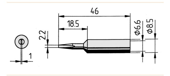
• Continuous soldering tip, straight, chisel-shaped, 2.2 mm wide, with ERSADUR-LF coating (lead-free soldering) for increased service life.
