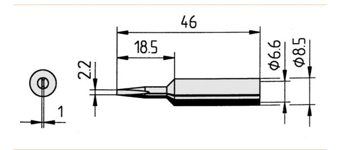
Continuous soldering tip, straight, chisel-shaped, 2.2 mm wide, with ERSADUR coating.
