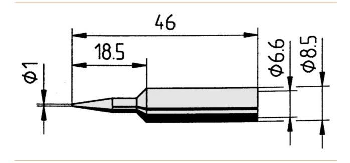
• Continuous soldering tip, straight, pencil tip, 1.0 mm diameter with ERSADUR-LF coating (lead-free soldering) for increased service life.
