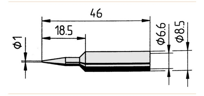
Continuous soldering tip, straight, pencil tip, 1.0 mm diameter, with ERSADUR coating.
