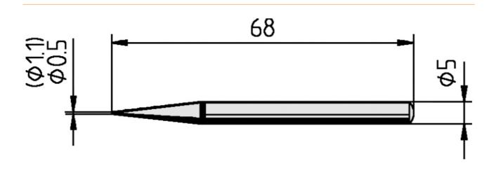
Continuous soldering tip for ERSA 30 S
