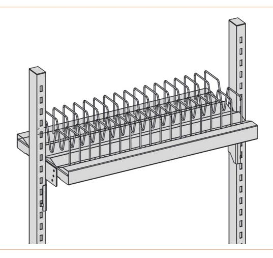
The hook-in storage board for SMD reels offers an efficient solution for storing SMD reels with diameters of 320 mm or 180 mm. Equipped with 35 dividers, it enables an orderly and clear arrangement of the reels. The board has a width of 860 mm and fits perfectly in CARs with a width of 970 mm, ensuring optimum use of space. A practical and flexible solution for organizing SMD reels in your working environment. We also offer matching dividers.
