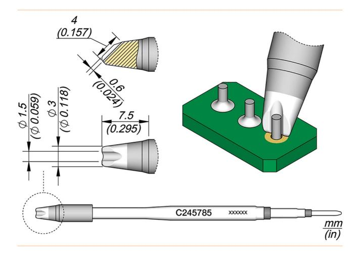
Soldering tips series C245 for soldering iron T245 (formerly AD-2245). They are suitable for general soldering purposes. Sleep and sleep mode in the clipboard. grooved
